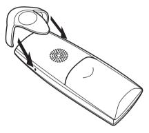
Attach the battery to the phone as shown in the figure below.
